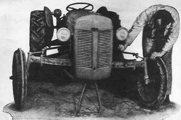
Adjusting front wheel tread width.
